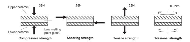
b) If a load is applied to the entire surface by a hard component, bending stress may be generated and the package may fracture, etc., depending on the flatness of the ceramic portions. Therefore, for installation, use either an elastic load, such as a spring plate, or an adhesive.
