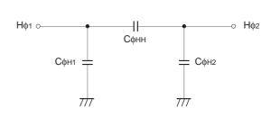
Vertical transfer clock equivalent circuit
